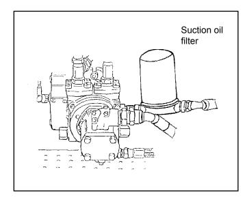
The **suction oil filter** is to be changed every 400th hour running. The suction oil filter is installed on the left of the engine house. Change the filter when the machine is cold. Screw off the filter by turning it counter-clockwise. Moisten the gasket of the new filter with oil and screw it on by hand. Do not tighten too hard.
